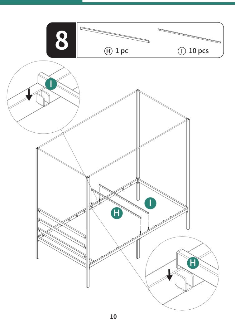
H-type steel slats can be installed into any side groove and provide solid support for the bed frame.
