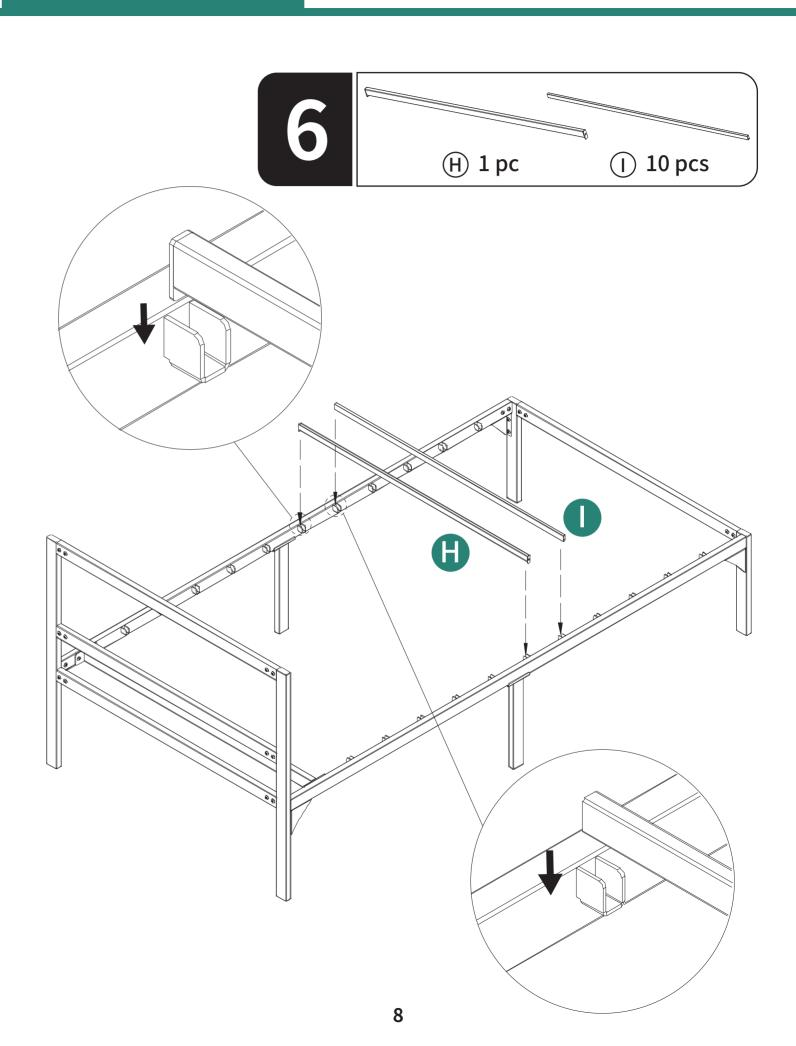
H-type steel slats can be installed into any side groove and provide solid support for the bed frame.
