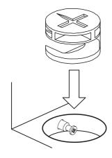
Turn the cam lock clockwise to tighten.
