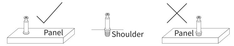
The pre-inserted nut should align with the center of the cam lock when joining two panels. The cam lock should be inserted before the eccentric wheel.
