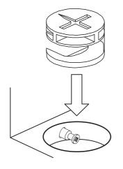
Turn the cam lock clockwise to tighten.
