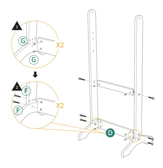
Attention: When installing Part A in step 3, it should be located in front of Part C and Part D without holes.
