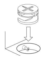
Turn the cam lock clockwise to tighten.
