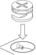
Turn the cam lock clockwise to tighten.
