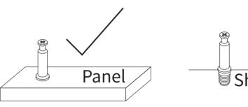
The pre-inserted nut should align with the center of the cam lock when joining two panels. The cam lock should be inserted before the eccentric wheel.
