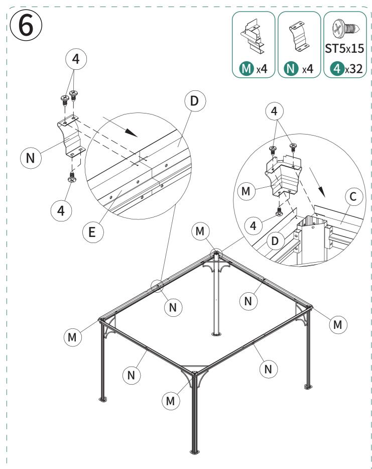
Finish connecting beams using corner covers (M) and screws I as shown in diagram. Affix middle beams using joint cover (N) and screws #4 as shown in diagram.
