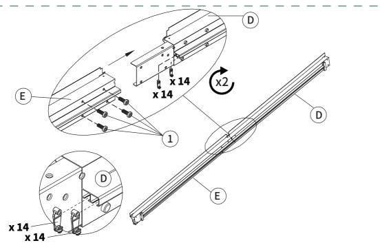
Put 28 Hooks (V) to each slot of sidewall track (D and E). Connect D and E into one beam using screws #1.
