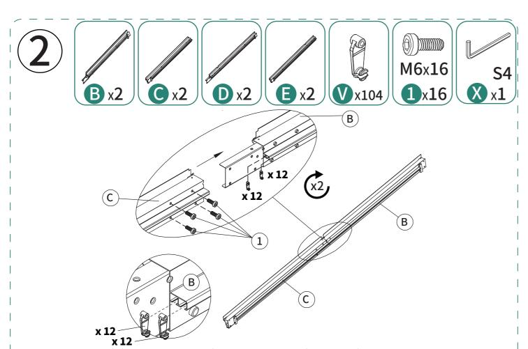
Put 24 Hooks (V) to each slot of sidewall track (B and C). Connect B and C into one beam using screws #1.
